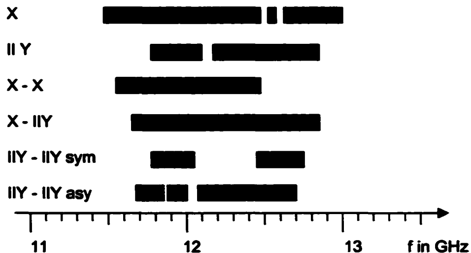
Figure 6.5: Frequency response of Type X and Type II Y waveguides and bends.
